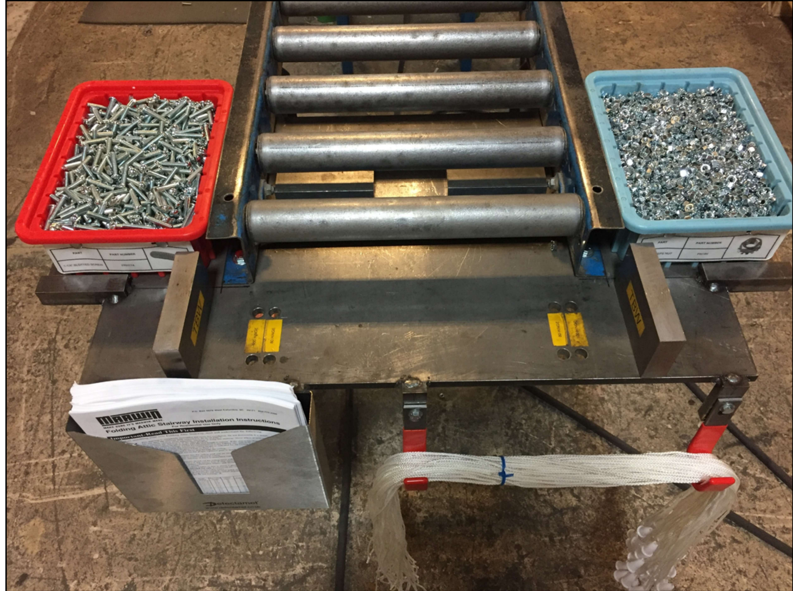
I later went on to mount the totes that contained the screws and bolts to the support rail base plate and pull cord hooks and instructions manual holder.
