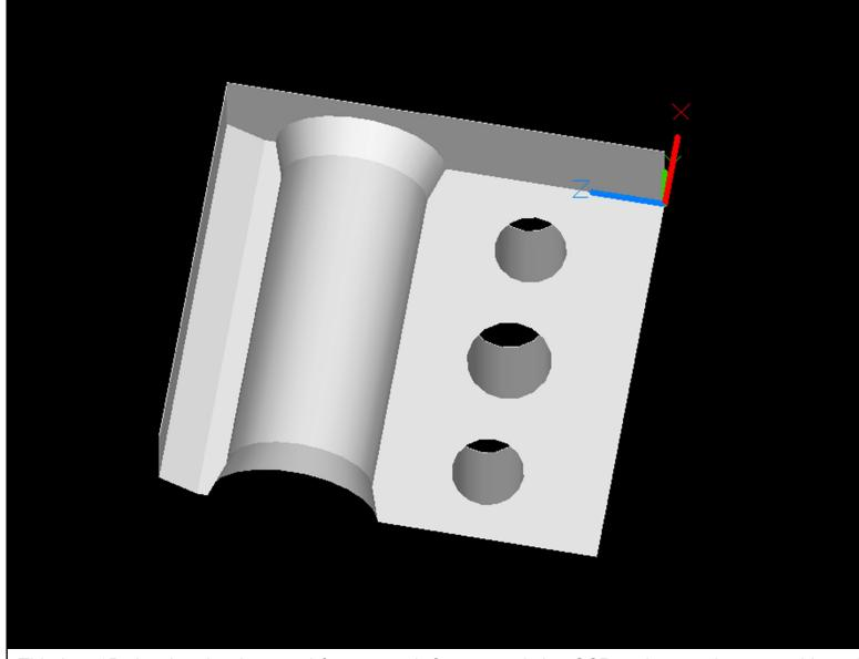
This is a 3D drawing that I created from scratch from an existing SCR tank vent pipe assembly tooling clamp serving as a template using AutoDesk AutoCAD 2D 3D 2024.
