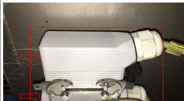
(ARROWED) HELIUM LEAK TESTER MULTI PIN ELECTRICAL LATCHING CONNECTOR (PLUG AND RECEPTACLE) I AM REQUESTING X10 REPLACEMENT HELIUM LEAK TESTER MULTI PIN ELECTRICAL LATCHING CONNECTOR PLUGS. AS THIS CONNECTS THE ELECTRICS FROM THE FIXTURE TO THE MACHINE. I AM CLASSIFYING THIS PART UNDER A FIXTURE. SPARE PART. I CANNOT MAKE OUT WHO THE MANUFACTURER IS AND ALMOST CERTAINLY A EUROPEAN MADE. WHAT HAS HAPPENED TO MANY OF THE CONNECTORS IS THAT THE LATCHING CLIPS HAVE BROKEN MAKING DIFFICULT FOR THE OPERATOR TO LATCH THE CONNECTOR IN PLACE. I AM ONLY REQUESTING THE RECEPTACLES BUT IF IT HAS TO COME WITH THE PLUG, I WILL HAVE TO PURCHASE THOSE TOO AS A SET IF NEED BE.
