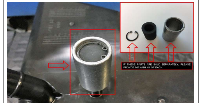
(ARROWED) HELIUM LEAK TESTER MBUSI VS30 SCR TANK CAP (PLUG) I AM REQUESTING X6 REPLACEMENT HELIUM LEAK TESTER MBUSI VS30 SCR TANK CAP (PLUG). THIS PLUG IS USED TO PLUG OR BLANK OFF A BARB FITTING ON THE SCR TANK DURING HELIUM LEAK TESTING. IF THIS IS A THREE (3) PART COMPONENT OF THE ALUMINUM CAP, SNAP RING (CIRCLIP) AND RUBBER PLUG OR BUNG PLUG THEN I WOULD LIKE TO HAVE SIX (6) OF EACH.
