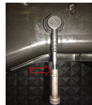
(ARROWED) HELIUM LEAK TESTER MBUSI VS30 SCR TANK PLUG ) I AM REQUESTING X6 REPLACEMENT HELIUM LEAK TESTER MBUSI VS30 SCR TANK TAPER PLUG. THIS PLUG IS USED TO PLUG OR BLANK OFF THE SO CALLED "VALVE" LOW FLOW WITH MEMBRANE DURING HELIUM LEAK TESTING. I AM SURE THIS M6 X 45 MM ALLEN CAP SCREW THAT LOOKS LIKE IT HAS BEEN TURNED DOWN ON THE END FOR A MAKE SHIT PLUG CAN NOT BE THE ORIGINAL DESIGN. PLEASE COULD YOU CHECK YOUR RECORDS OF WHAT THE ORIGINAL DESIGN WAS AND SEND THOSE TO ME.
