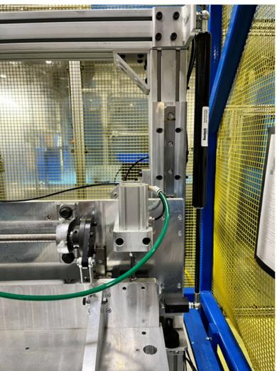
Picture showing left hand side and right hand side air cylinders at either end of cam shaft to operate in tandem for equal force.
