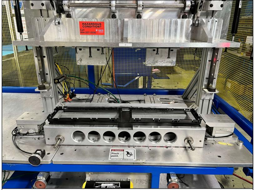
This is a semi-automatic assembly machine that assembles the front AGS (Active Grill Shutter) front frame to the vane body on the Honda MDX program vehicle.
