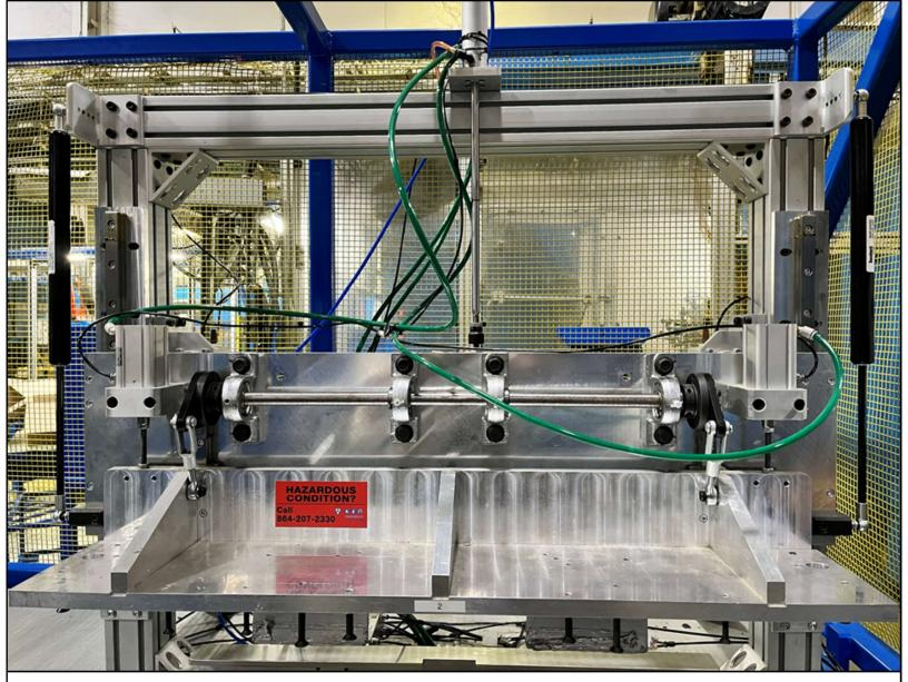
The press is powered by two SMC 50  $\emptyset$  mm X 125 mm air cylinders linked together by a cam shaft to provide equal downward force, but it wasn't enough.
