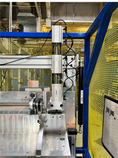
This picture shows both left hand and right hand all three (3) cylinders installed stacked on top of one another connected together by their piston rods.
