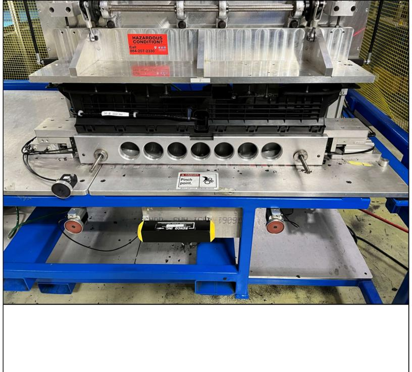
UPPER PRESS LOWER INTO POSITION ON TOP OF THE VANE BODY AND PRESSURE APPLIED
