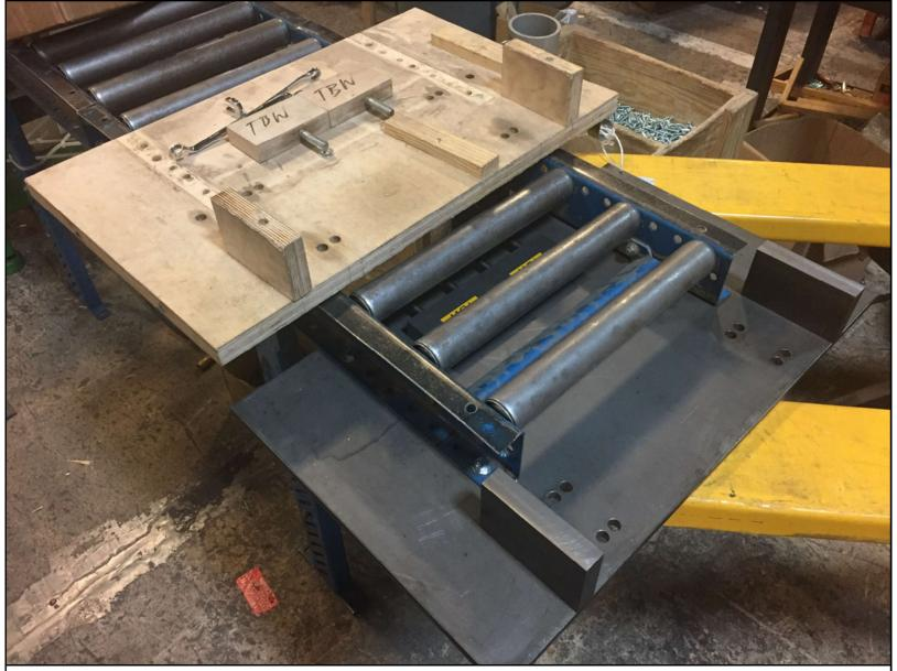
This picture shows both my original mock up design made from wood and my later design made from steel.
