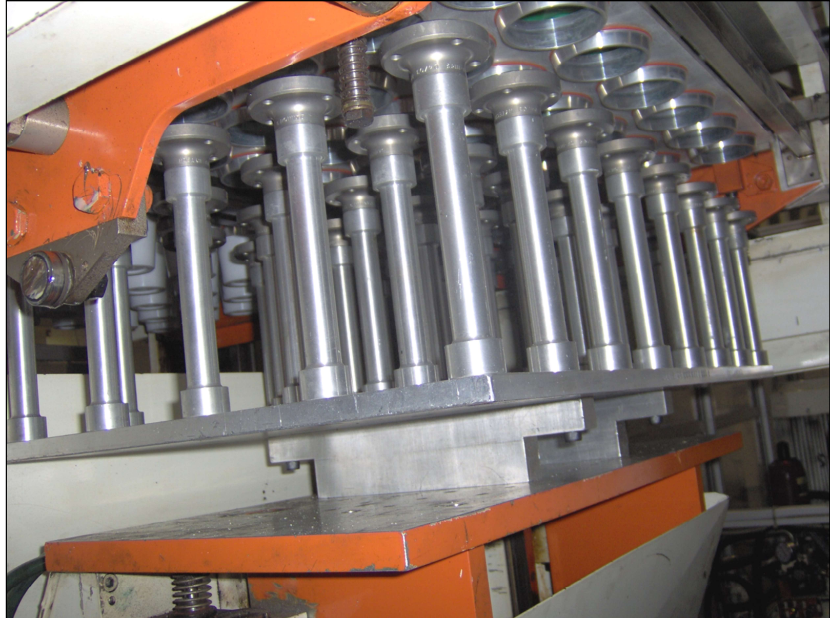
Picture showing the lifting station through the transfer plate.
