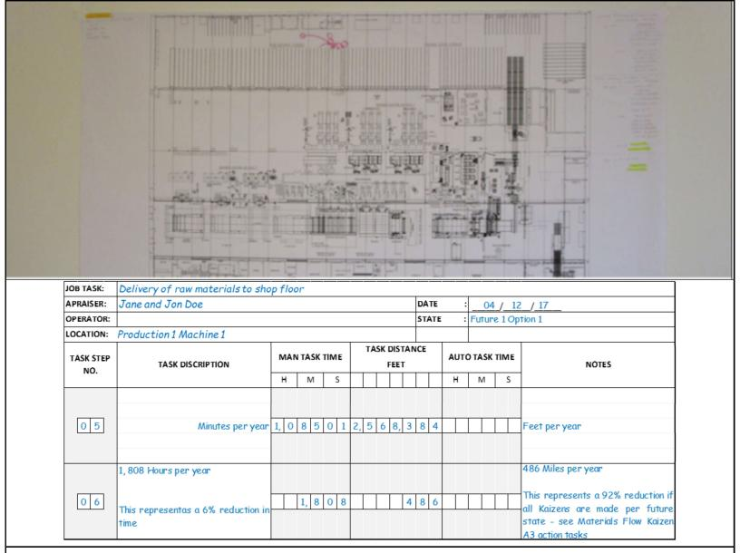
This was the Future State Map of taking raw bales materials from warehouse location to the side line storage location. Extrapolated distance per year 400 miles. This does involve the capital project of installing a gravity feed conveyor through the partition wall to the pick point line side storage potentially resulting in a 92% reduction in distance.
