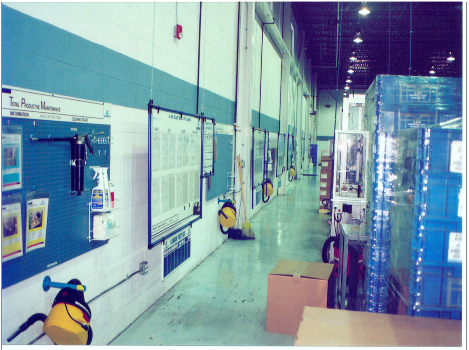
Picture showing TPM pegboards that I installed for each production line where individualized components such as grease guns, hand tools, high frequency use and expendable parts were stored.
