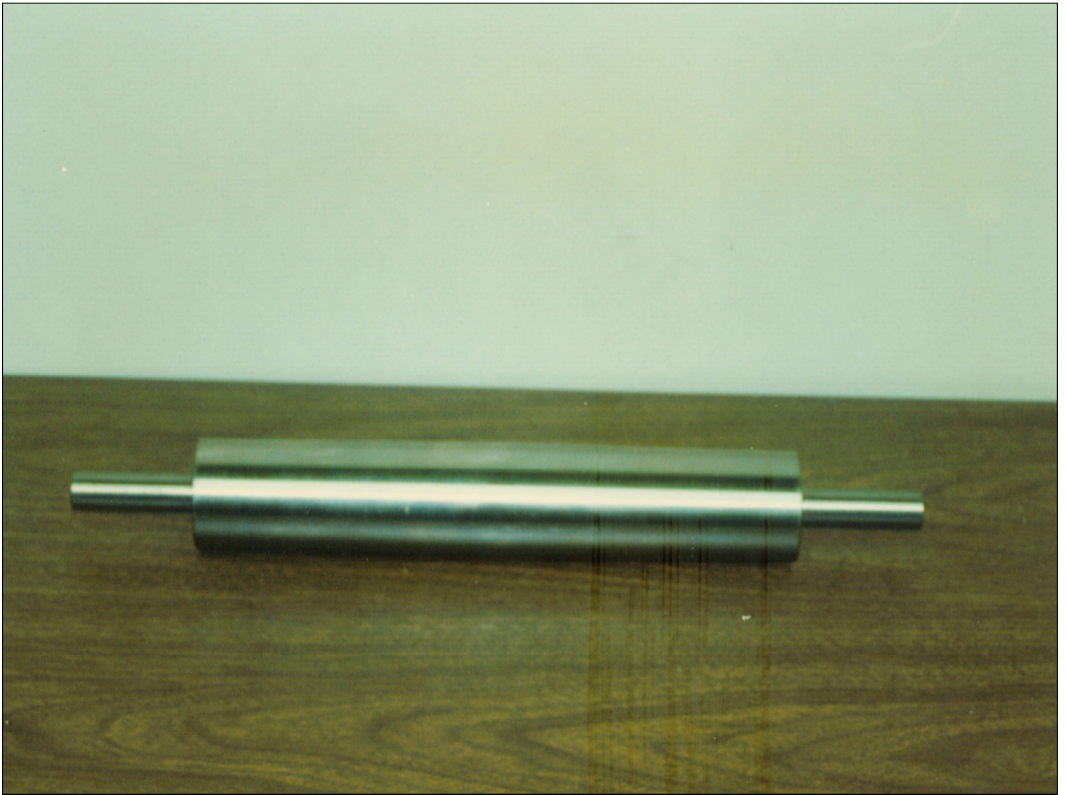
Pictures showing replacement conveyor idler roller.
