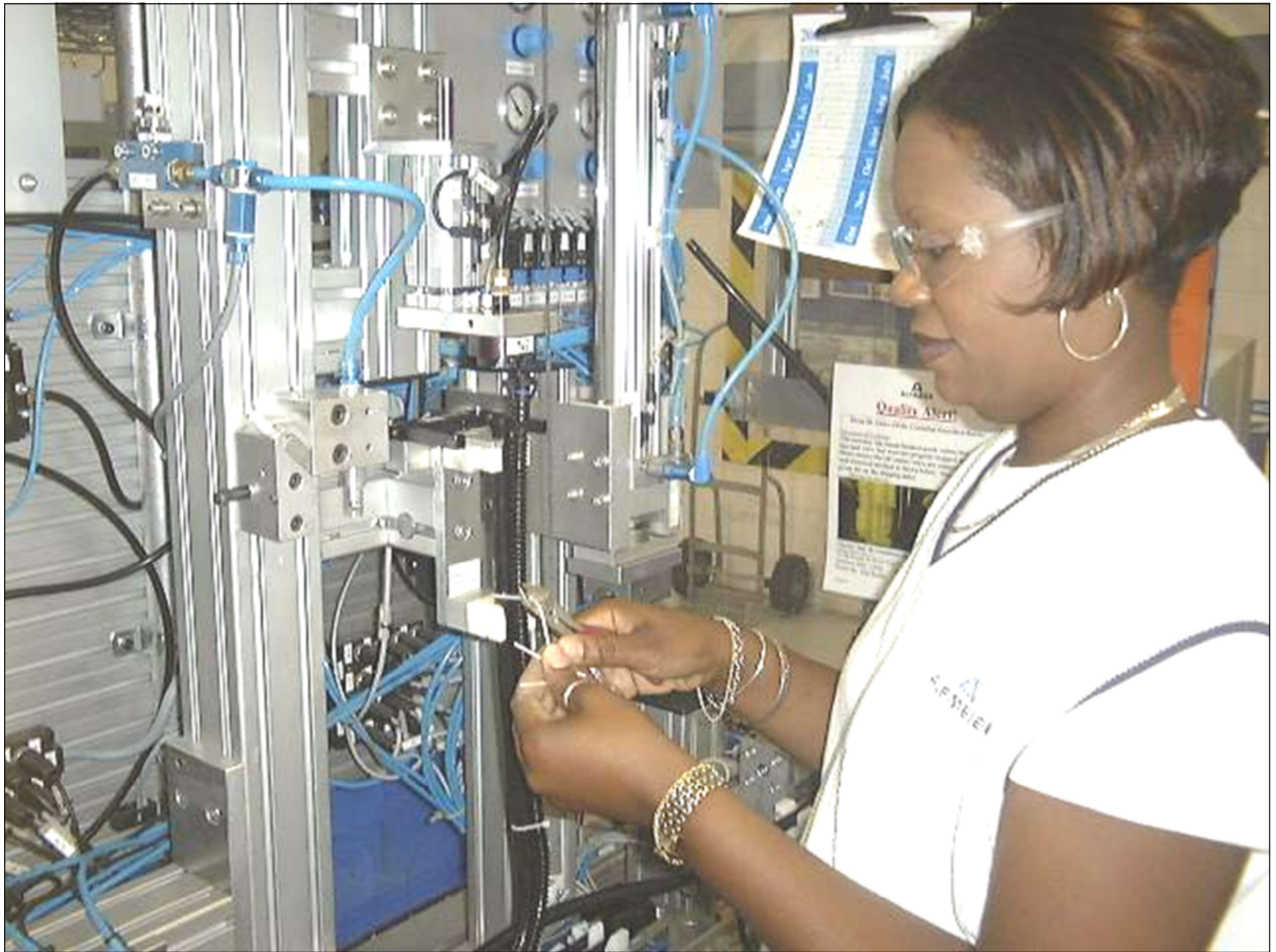
Picture showing the operator using the side cutters to remove excess length from cable ties installed on this part in the final process of assembly.
