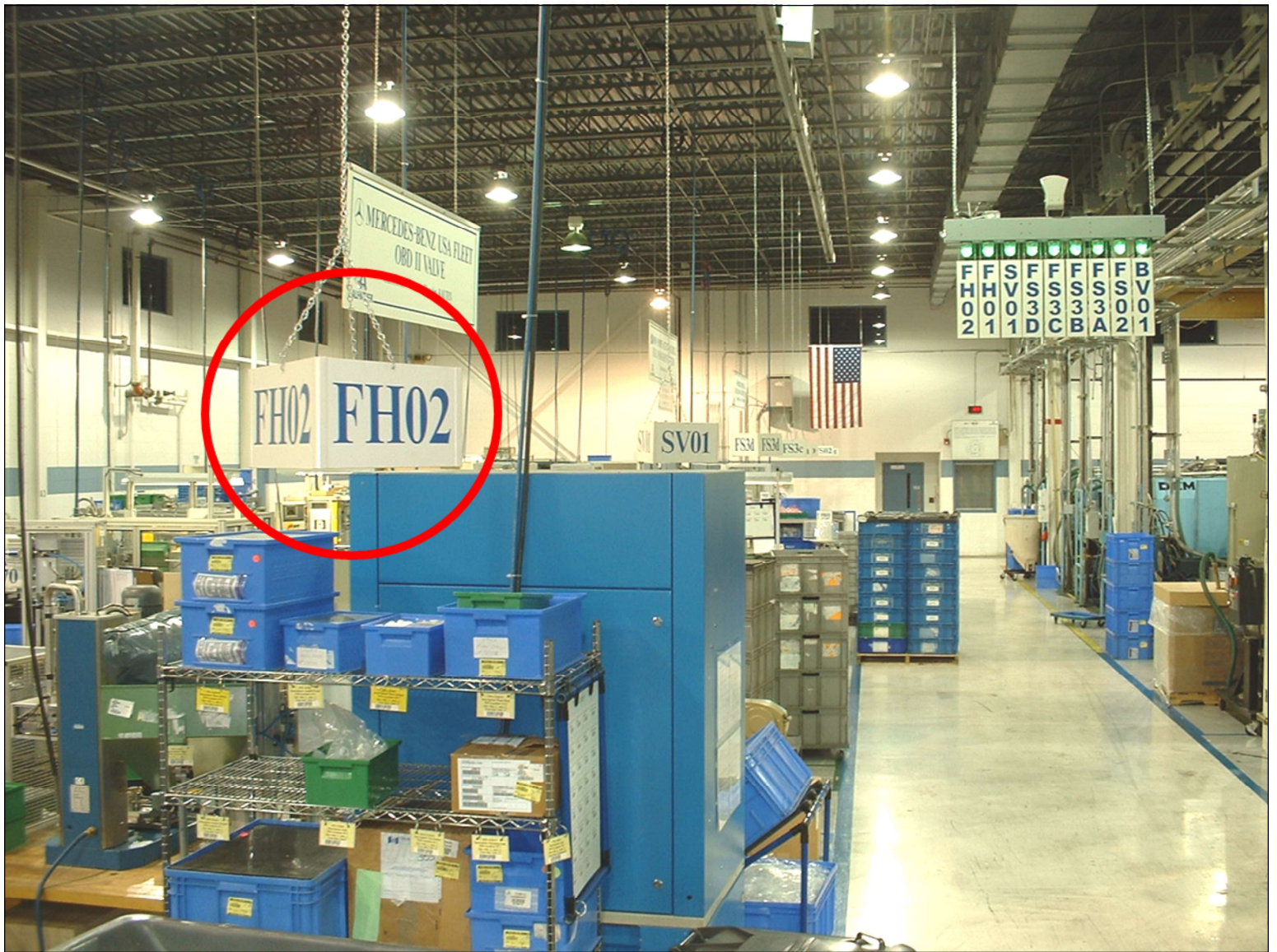
5S visual management... Example of a triangle signboard, done so that it can be seen from any direction.
